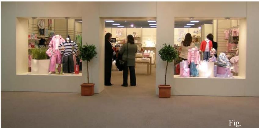
Each Window had 2 No. 70W Feature lights in the ceiling above the display and 3 No. adjustable 12V 50W dichroic fittings on the floor of the display.
